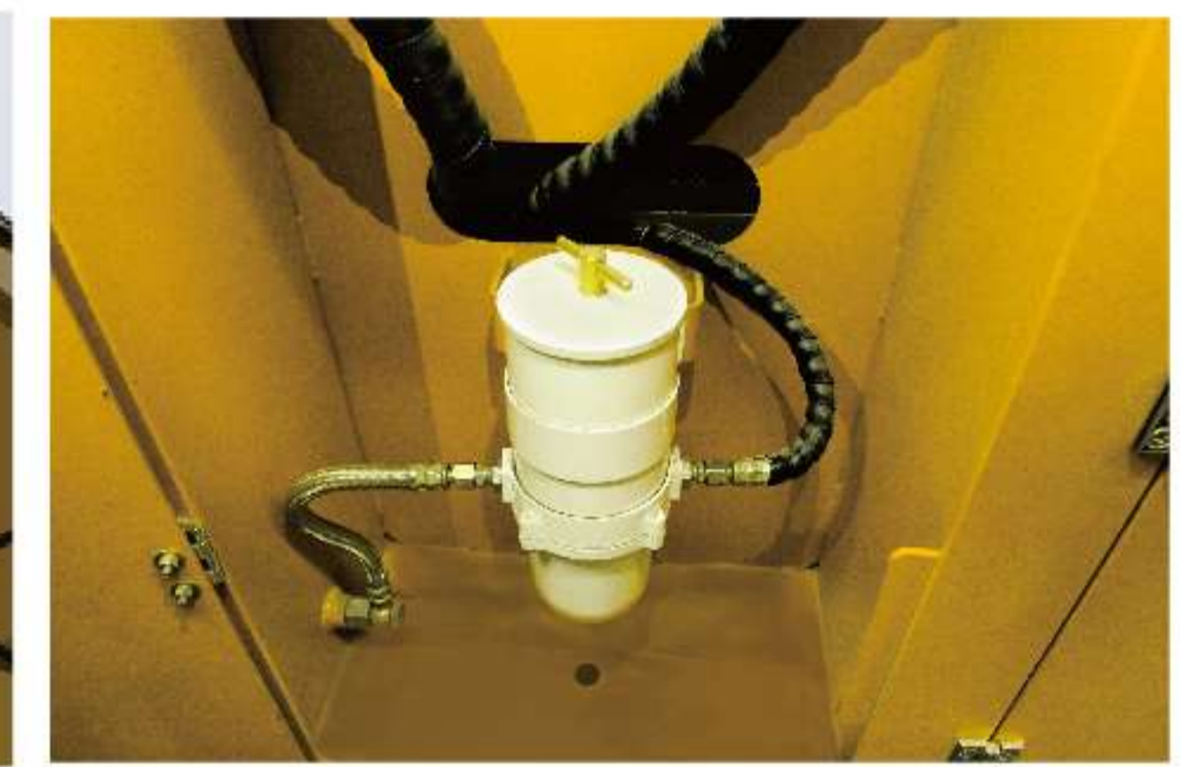
▪ Steel wire winded hoses are used and safety level is improved greatly.
