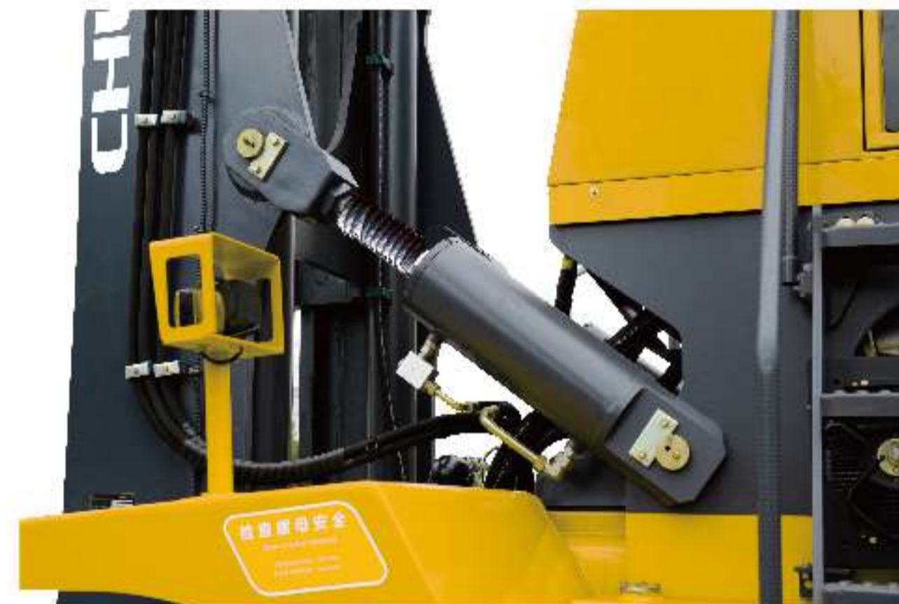
▪ Oil cylinder protection sleeve(optional): it is used to protect cylinder damaged from foreign matters
