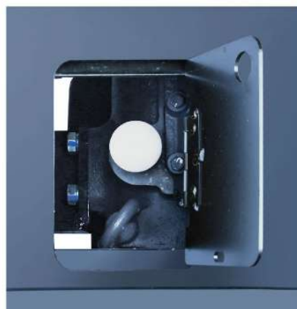
Floor board with checking hole, which is convenient to gearbox maintenance.
