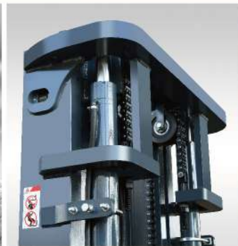
Frame type upper beam, more reasonable structure, enhance the rigidity and strength
