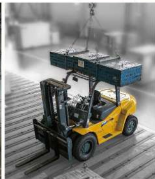
Impact test of overhead guard
